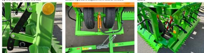
detail: mechanical adjustment of triangle board hydraulically adjustment 1st triangle board by the switcher from the cab
